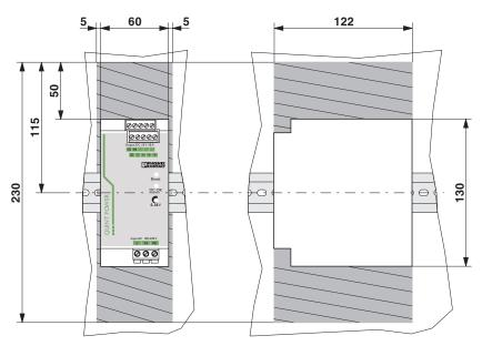
Slim-style installation: Installation depth 125 mm (+ DIN rail)
