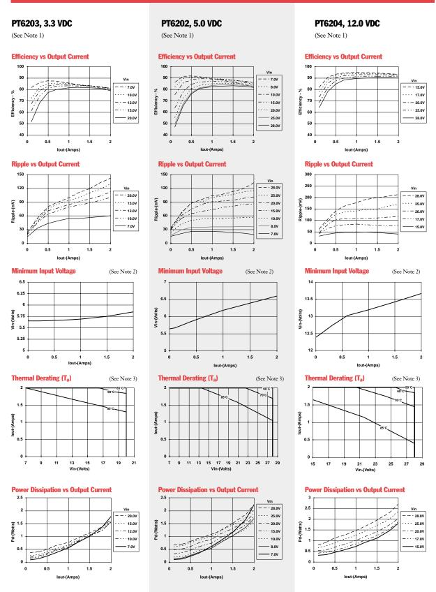
Note 1: All data listed in the above graphs, except for derating data, has been developed from actual products tested at 25°C. This data is considered typical data for the ISR. Note 2: Minimum  $V_m$  data is typical and is not guaranteed. The data corresponds to a 2% output voltage drop.
