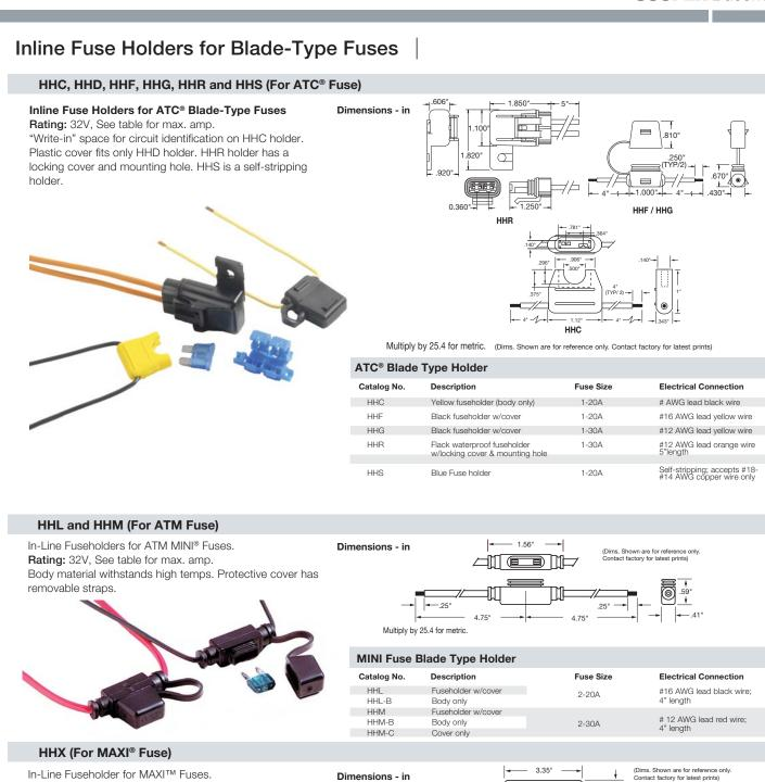
In-Line Fuseholder for MAXI™ Fuses. **Rating:** 32V, 60A Max. Firewall mounting hole permits two or more holders to be mounted together. Cover comes with a removable strap.
