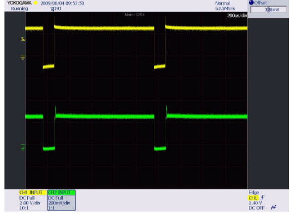
V_{IN} = 4.2\text{ V} , Ch1 – EN/SET, Ch2 – LED current (400 mA/div)
