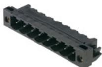
High-temperature-resistant male connector, packed in box or tape. In tape with 1.5 mm solder pin optimised for automatic assembly. 3.2 mm solder pin suitable for reflow and wave soldering. These male connectors can be labelled and coded.
