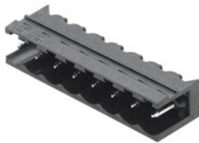
High-temperature-resistant, 90° angled, open male connector. Packed in box or tape. In tape with 1.5 mm solder pin optimised for automatic assembly. 3.2 mm solder pin suitable for reflow and wave soldering. These male connectors can be labelled and coded.
