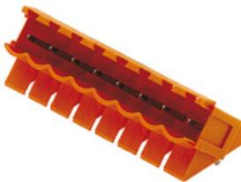
Male connectors with 135° outlet direction. The solder pin length is optimised for wave flow soldering. The male connectors provide space for labelling and can be coded. Packed in cardboard box.
