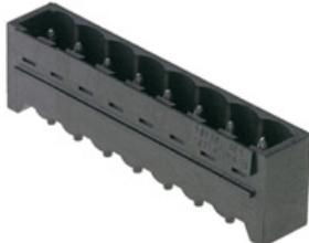
High-temperature-resistant male connector, packed in box or tape. In tape with 1.5 mm solder pin optimised for automatic assembly. 3.2 mm solder pin suitable for reflow and wave soldering. These male connectors can be labelled and coded.
