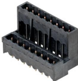
High-temperature resistant, double level, laterally offset, closed ended male connector, with solder flange option. 1.5 mm solder pin suitable for reflow soldering. 3.2 mm solder pin suitable for reflow and wave soldering. These male connectors can be labelled and coded. Packed in cardboard box.
