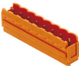
Male connectors with straight outlet direction. The solder pin length is optimised for wave flow soldering. The male connectors provide space for labelling and can be coded. Packed in cardboard box.
