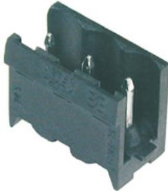
High-temperature-resistant male connector for side-by-side mounting. Packed in tape with 1.5 mm solder pin. Optimised for automatic assembly and suitable for reflow soldering. These male connectors can be labelled and coded.
