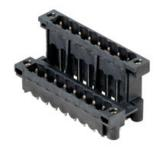
High-temperature resistant, double level, laterally offset, closed ended male connector, with solder flange option. 1.5 mm solder pin suitable for reflow soldering. 3.2 mm solder pin suitable for reflow and wave soldering. These male connectors can be labelled and coded. Packed in cardboard box.
