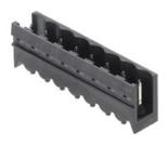
High-temperature-resistant, straight, open ended male connector. Packed in box or tape. In tape with 1.5 mm solder pin optimised for automatic assembly. 3.2 mm solder pin suitable for reflow and wave soldering. These male connectors can be labelled and coded.
