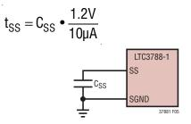
Figure 5. Using the SS Pin to Program Soft-Start
