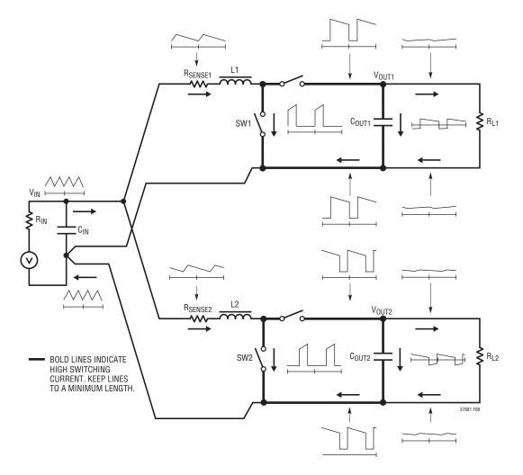
Figure 8. Branch Current Waveforms
