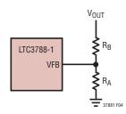
Figure 4. Setting Output Voltage
