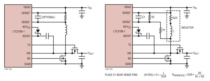
(2a) Using a Resistor to Sense Current
