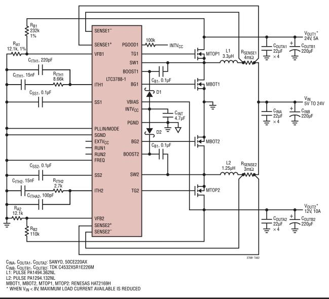
High Efficiency Dual 12V/24V Boost Converter
