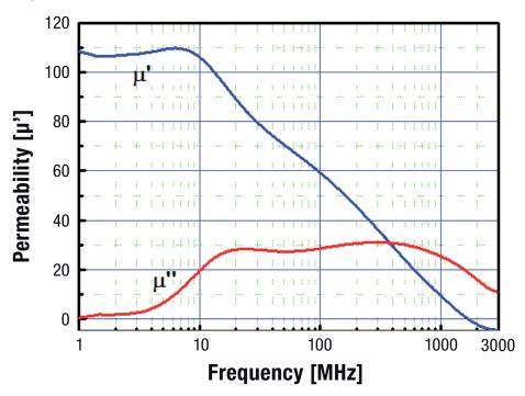
$<sup>^2</sup>$ Attenuation is measured by 7mm coaxial verification kit under short fixed condition. Power loss is measured by a 50Ω microstrip line method. 3M TM K-RD-EMC-AB-01.
