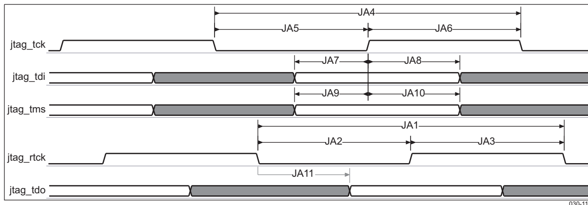
Figure 6-73. JTAG Interface Timing – Adaptive Clock Mode
