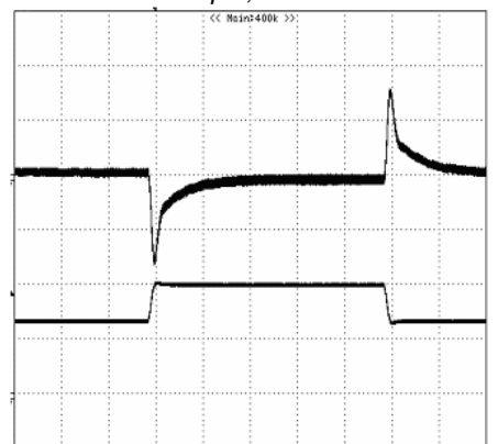
Figure 8: Output voltage response to step-change in load current (75%-50%-75% of I_o , max; di/dt = 0.1A/\mu s ). Load cap: 10 \mu F tantalum capacitor and 1 \mu F ceramic capacitor. Top Trace: V_{out} (100mV/div, 200us/div), Bottom Trace: I_{out} (2A/div). Scope measurement should be made using a BNC cable (length shorter than 20 inches). Position the load between 51 mm to 76 mm (2 inches to 3 inches) from the module
