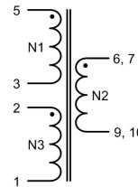
N2 is made of two bifilar windings. Therefore customer has to tie terminals 6+7 and 9+10 on PCB. A general separation of the two windings cannot be guaranteed.
