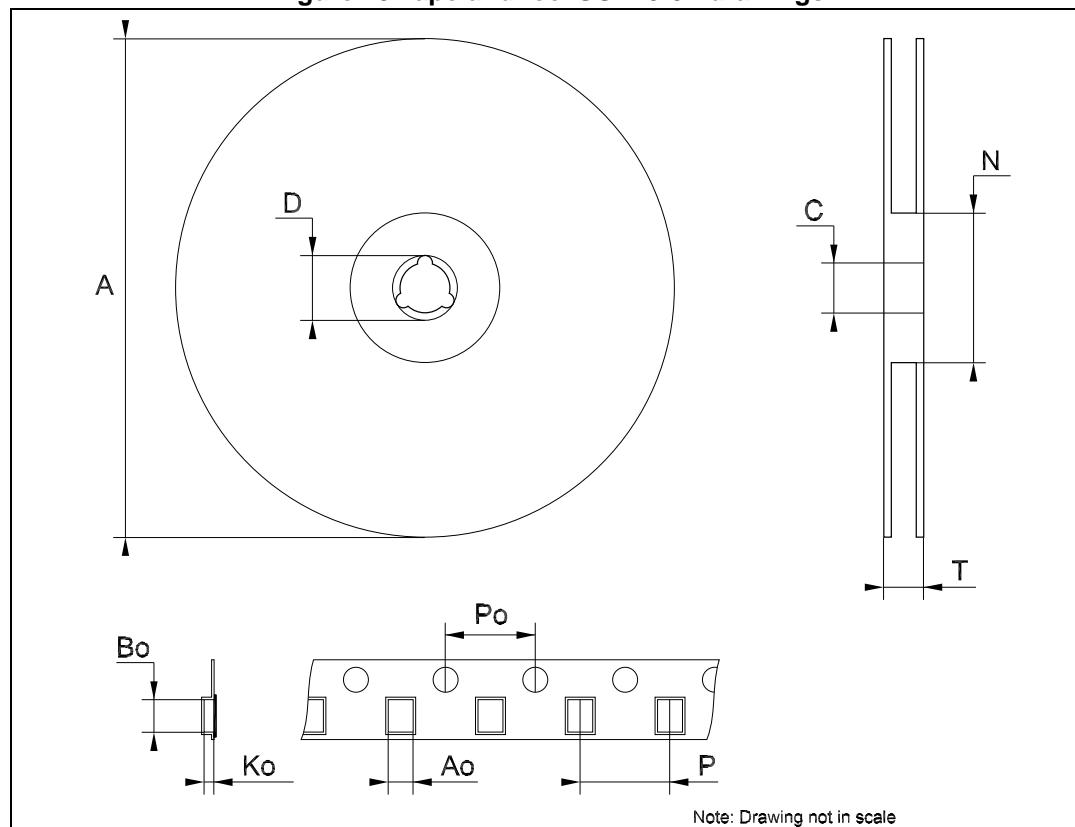
Table 7. Tape and reel SOT23-5L mechanical data
