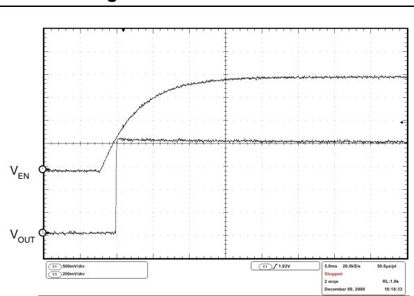
V<sub>IN</sub> = 1.5 V; V<sub>EN</sub> from 0 to 2 V, no load, T = 25 °C
