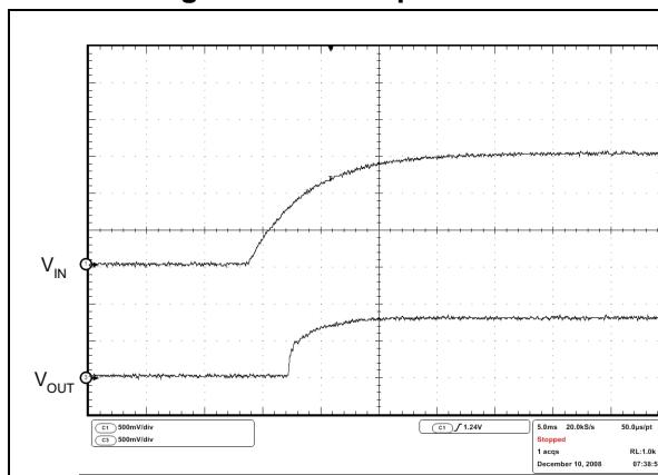
V<sub>IN</sub> from 0 to 1.5 V, V<sub>EN</sub> tied to V<sub>IN</sub>, no load C<sub>OUT</sub> = 1 µF
