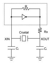
$C_L = 2^*(C_P - C_S),$  Where  $C_P =$  Load capacitance of crystal from crystal vendor datasheet.
