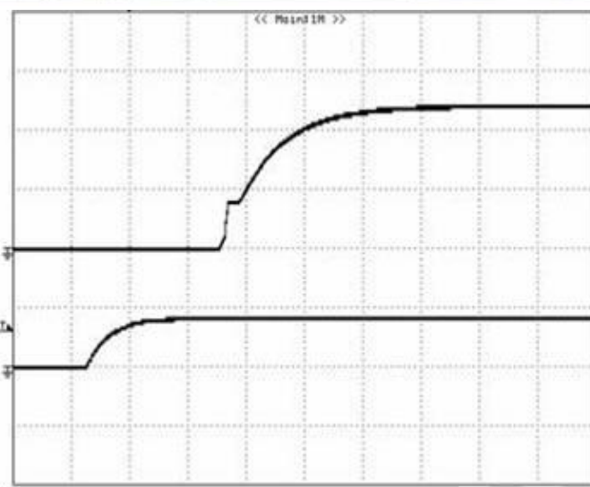
Figure 6: (For positive remote on/off logic) Turn-on transient at full rated load current (5 ms/div). V_{in}=48V . Top Trace: V_{out} , 5V/div, Bottom Trace: ON/OFF input, 5V/div.
