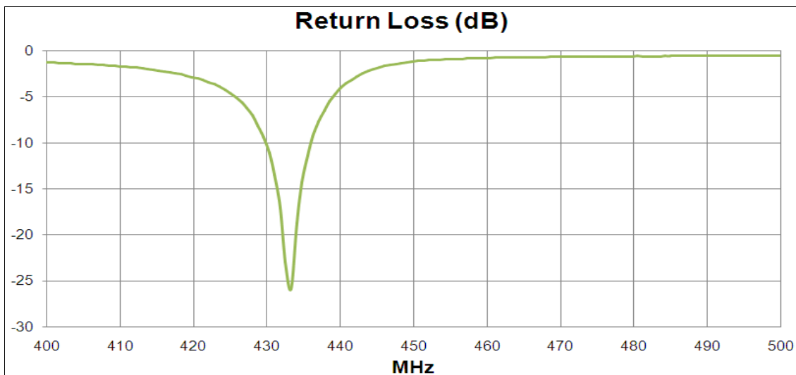
Figure 2. Return Loss for the FXP240 Antenna.
