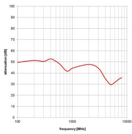
measurement based on assembeled top cover with THT frame according to IEEE STD 299
