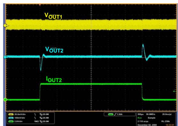
FIGURE 12. LOAD TRANSIENT: INPUT VOLTAGE = 18V, I_{OUT1} = 3A , I_{OUT2} = 0A \leftrightarrow 3A
