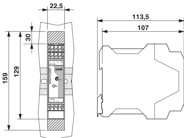
Mounting position: Installation depth 107 mm (+ DIN rail)
