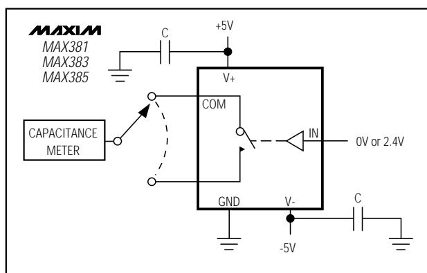
Figure 8. Channel-On Capacitance
