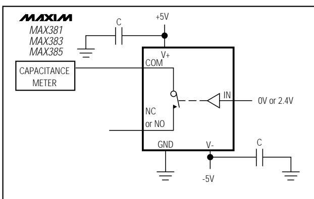
Figure 7. Channel-Off Capacitance
