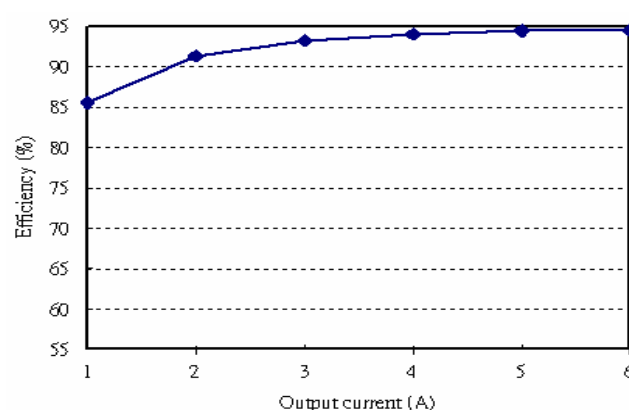
Figure 4: Converter efficiency vs. output current (2.5V output voltage, 12V input voltage)
