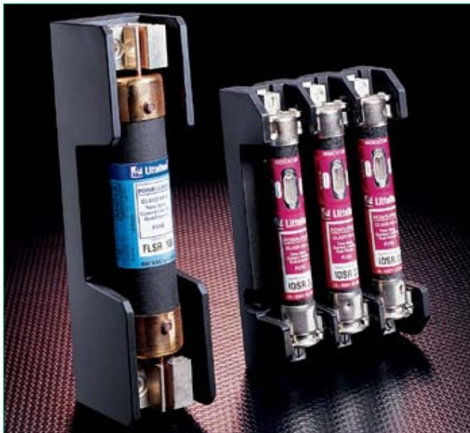
Class H and Class R fuse blocks are dimensionally the same, but Class R blocks incorporate a rejection feature, which only allows Class R fuses to be inserted.
