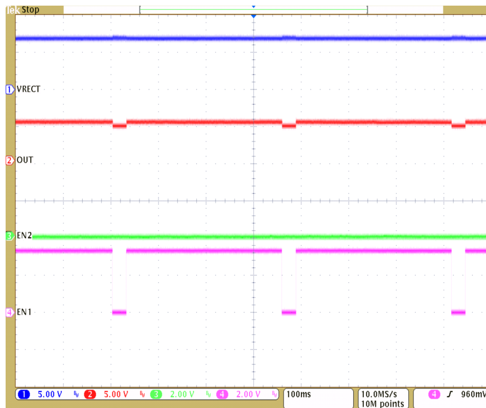
Figure 4. Utilizing Internal bq25046 Current Limit In a Wireless Power Application
