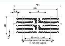
Pitch 5 mm a = Area for mounting components, 38 mm in the hood b = Area for mounting components, 45 mm in the housing
