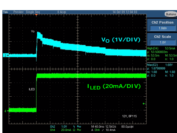
FIGURE 22. LOAD REGULATION WITH I_{LED} CHANGES FROM 0% TO 100% PWM DIMMING
