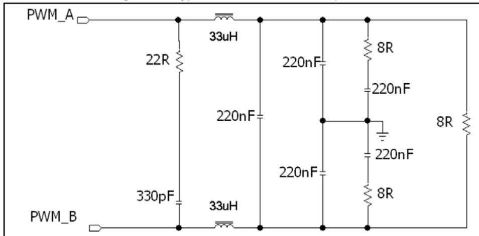
Figure 25: Typical LC filter for a 6 Ω speaker
