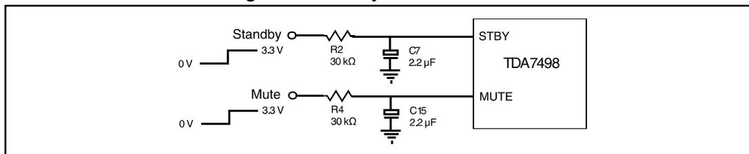
Figure 21: Turn on/off sequence for minimizing speaker "pop"
