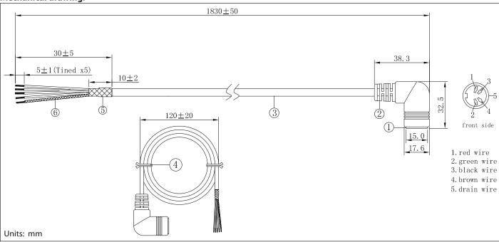
tolerance X: ±0.5 mm .X: ±0.3 mm .XX: ±0.05 mm applicable unless otherwise indicated in specification or on drawings Tensility International Corporation reserves the right to substitute parts which are functionally equivalent to the ones specified.
