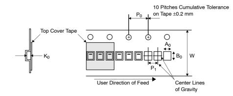
Figure 1. Tape and Reel Mechanical Data
