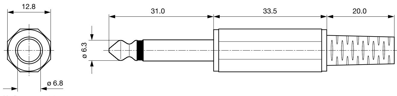
Cable diameter max. 6.8 mm
