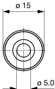
Cable diameter max. 5.0 mm
