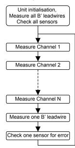
The leadwire compensation measurement and sensor error detection for each input are executed once every N cycles (N = number of active inputs)
