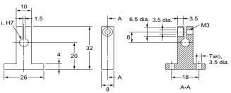
Tightening torque: 0.6 to 0.8 N•m (M3 screw)
