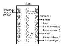
Note: Two inputs are possible on the K3AS, however, due to the output circuit of the D5SN, two current inputs are not possible.
