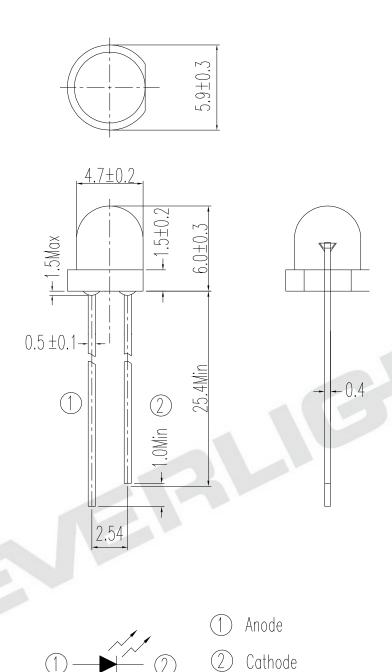
Note: Tolerances unless dimensions ±0.25mm
