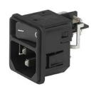
DC11, Mounting: Screw, Rocker switch: non-illuminated or illuminated 1 or 2 pole, Quick connect terminals 4.8 x 0.8 mm, Appliance Inlet: IEC C14, Without fuse holder: Suitable for appliances with protection class I or II
