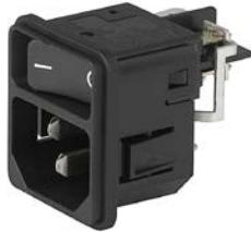
DC11, Mounting: Screw, Rocker switch: non-illuminated or illuminated 1 or 2 pole, Quick connect terminals 4.8 x 0.8 mm, Appliance Inlet: IEC C14, Without fuse holder: Suitable for appliances with protection class I or II
