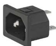
6010, Mounting: Snap-in, Solder, quick-connect, screw, PCB, Appliance Inlet: IEC C14
