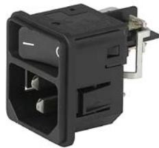
DC11, Mounting: Screw, Rocker switch: non-illuminated or illuminated 1 or 2 pole, Quick connect terminals 4.8 x 0.8 mm, Appliance Inlet: IEC C14, Without fuse holder: Suitable for appliances with protection class I or II
