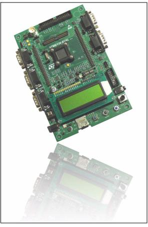
The full range of hardware features helps you to evaluate all peripherals (including motor control, CAN, micro SD Card, smartcard, UART, LIN, IrDA) and develop your own applications. Extension headers make it possible to easily connect a daughterboard or wrapping board for your specific application.
