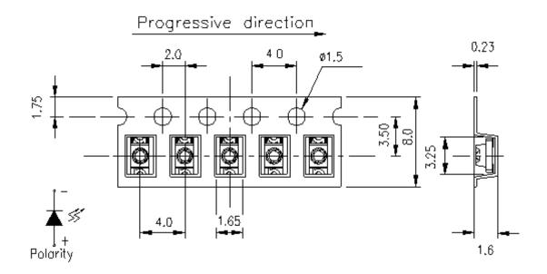
**Note:** The tolerances unless mentioned are  $\pm 0.1$ , Unit = mm.
