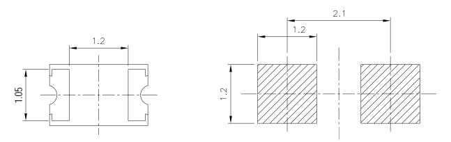
**Note:** The tolerances unless mentioned is  $\pm 0.1$  mm ,Unit = mm
