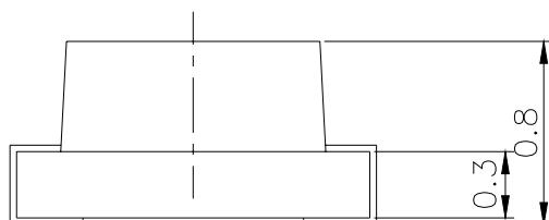
For reflow soldering (Propose)
