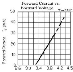
Forward Voltage VF(V)
