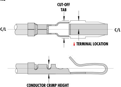
Iterminal is to be centrally located between the two (2) cut-off tab edges by one half of the total cut-off tab tolerance. This illustration is a generic terminal representation and not an exact image of any terminal listed in the scope.
