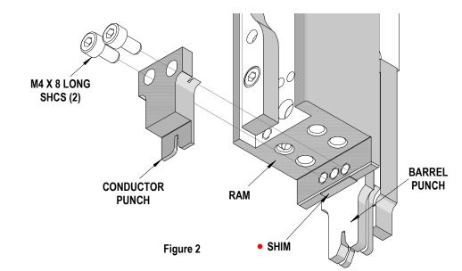
• Shim location for Conductor Punch. Shim size should be .38 by 3.2 by 12.7mm (.015 by 1/8 by 1/2").
