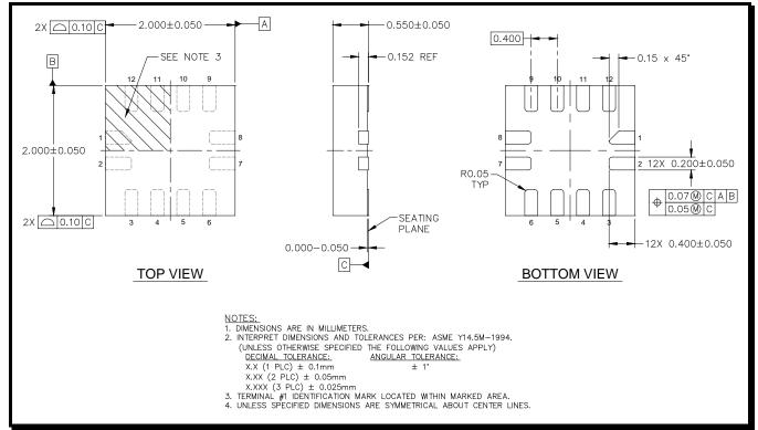
Figure 5: SE2601T Package Diagram
