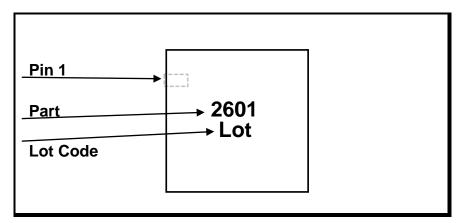
Figure 4: SE2601T Branding and Pin 1 Location
