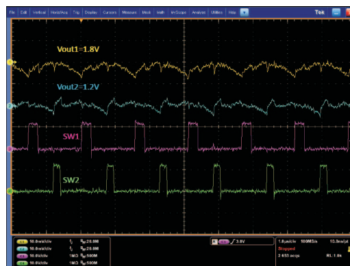
Figure 8. Buck 1 and Buck 2 in Steady State I_{O1} = 2\text{ A} , I_{O2} = 3\text{ A}
