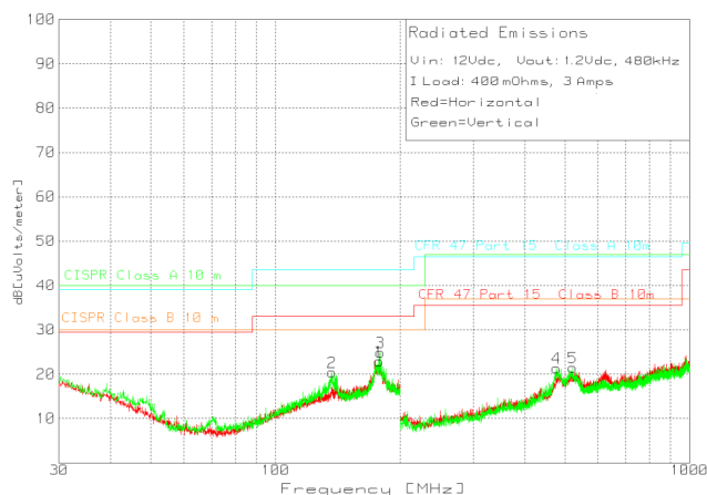
Figure 45. Radiated Emissions 12-V Input, 1.2-V Output, 3-A Load (EN55022 Class B)
