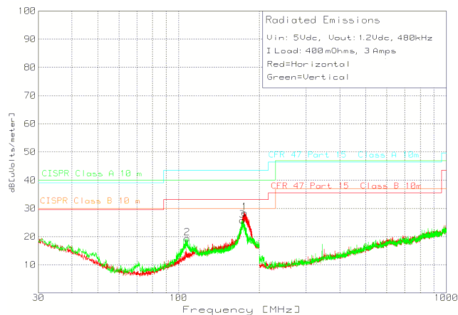
Figure 44. Radiated Emissions 5-V Input, 1.2-V Output, 3-A Load (EN55022 Class B)
