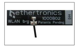
Ethertronics' Prestta series of Isolated Magnetic Dipole<sup>™</sup> (IMD) trace antennas address the challenges facing today's product designers. IMD's high performance and isolation characteristics offer better connectivity and minimal interference.
