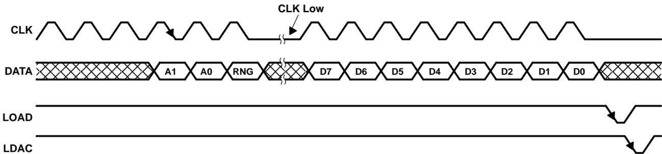
**Figure 4. LDAC-Controlled Update Using 8-Bit Serial Word**
