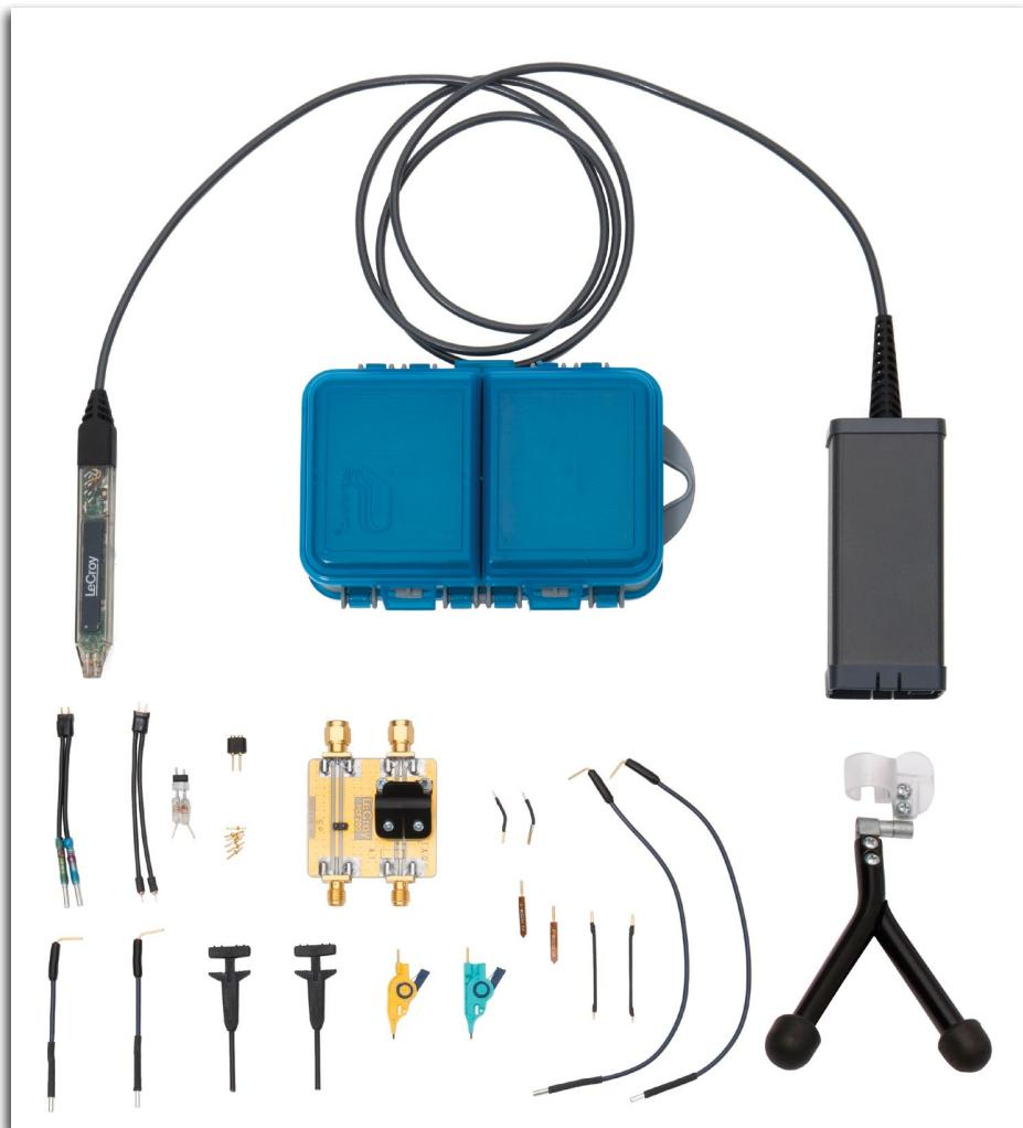
The differential input capacitance is only 1 pF to minimize loading distortion on the highest frequency signals under test. System noise of only 4 mV<sub>rms</sub> allows accurate measurement of the smallest signals.
