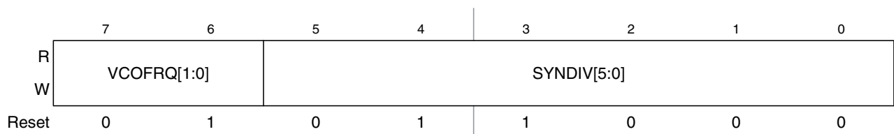
Figure 10-4. S12CPMU Synthesizer Register (CPMUSYNR)
