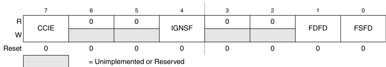
Figure 26-9. Flash Configuration Register (FCNFG)
